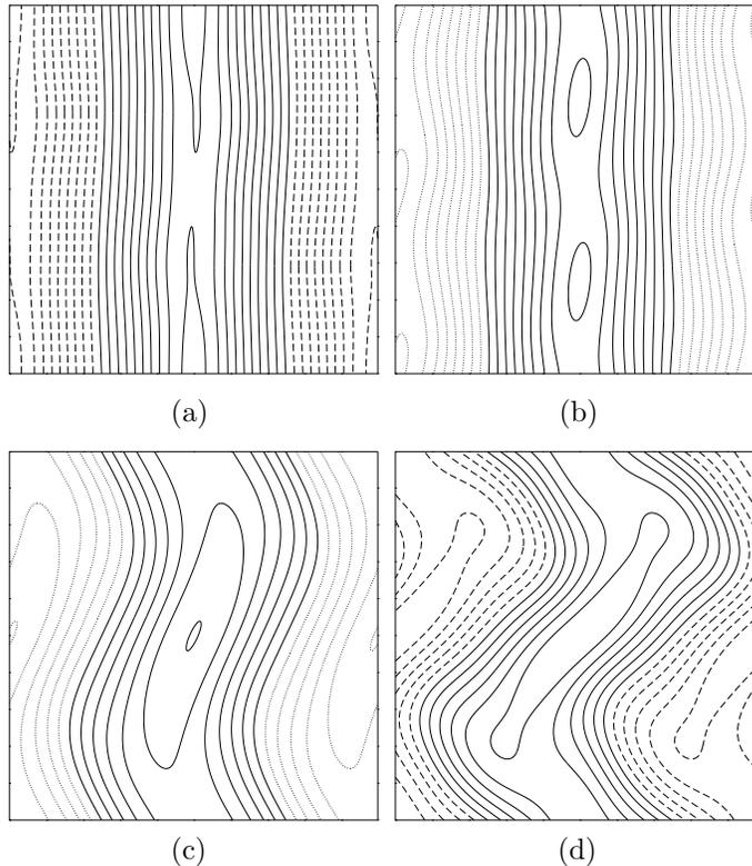
Figure 10: Isolines (step 2) of  $v_z$  on the horizontal midplane  $z = 1/2$  for some steady convective MHD attractors:  $S_1^{R1}$ ,  $Ta = 150$  (a);  $S_3^{R1}$ ,  $Ta = 250$  (b);  $S_8^{R1}$ ,  $Ta = 680$  (c);  $S^{WR}$ ,  $Ta = 721$  (d). Solid lines indicate non-negative, dashed lines negative values.  $x$ : horizontal axis,  $y$ : vertical axis.
