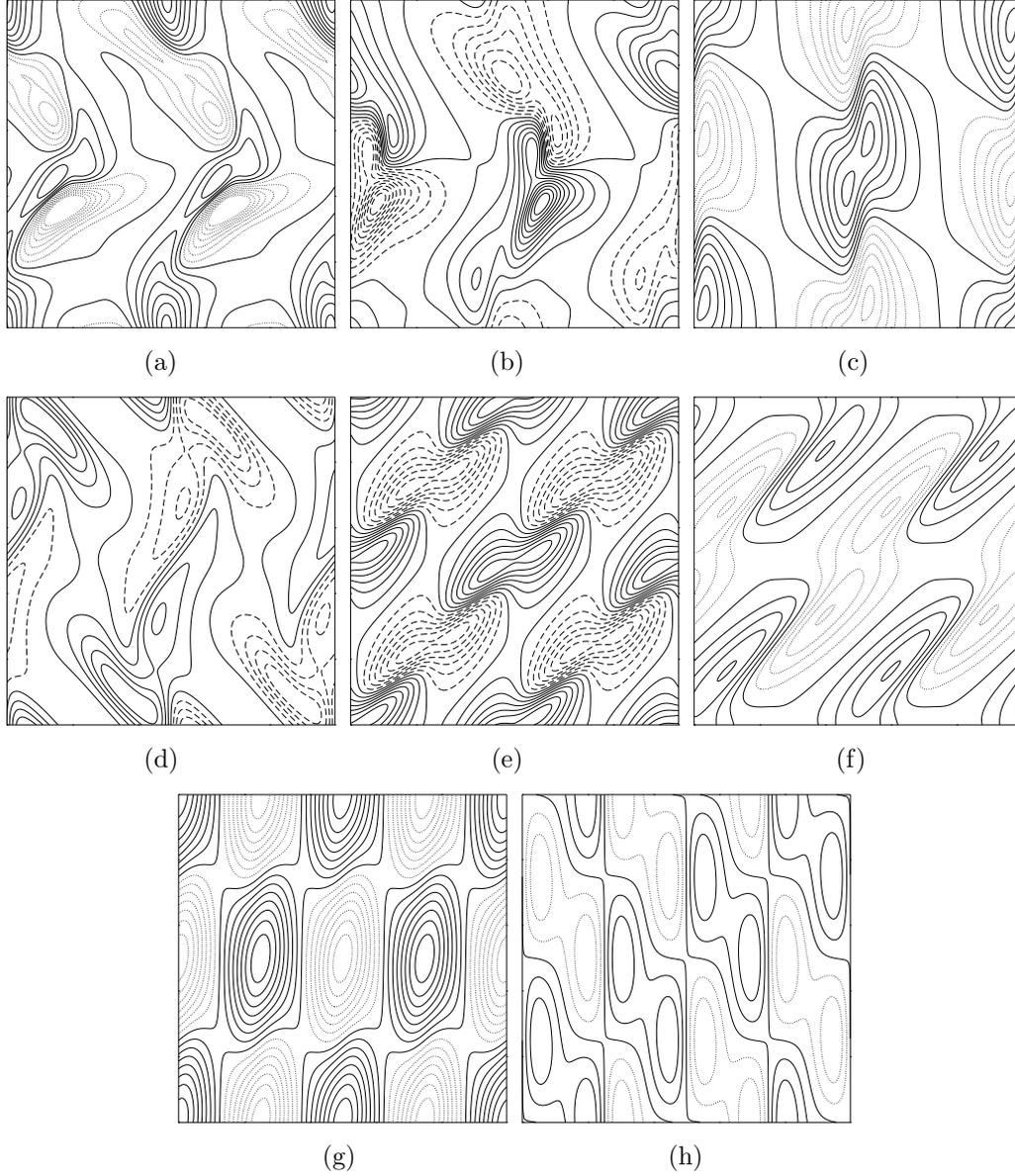
Figure 4: Isolines step 0.2 of  $b_z$  on the horizontal midplane  $z = 1/2$  for dominant magnetic modes:  $Ta = 50$ , TW (a);  $Ta = 150$ , TW (b);  $Ta = 500$ ,  $R_1$  (c);  $Ta = 720$ , WR (d);  $Ta = 685$ ,  $R_D$  (e);  $Ta = 1200$ ,  $R_D$  (f);  $Ta = 1100$ ,  $R_2$  (g);  $Ta = 1700$ ,  $R_2$  (h). Solid lines indicate non-negative, dashed lines negative values.  $x$ : horizontal axis,  $y$ : vertical axis.
