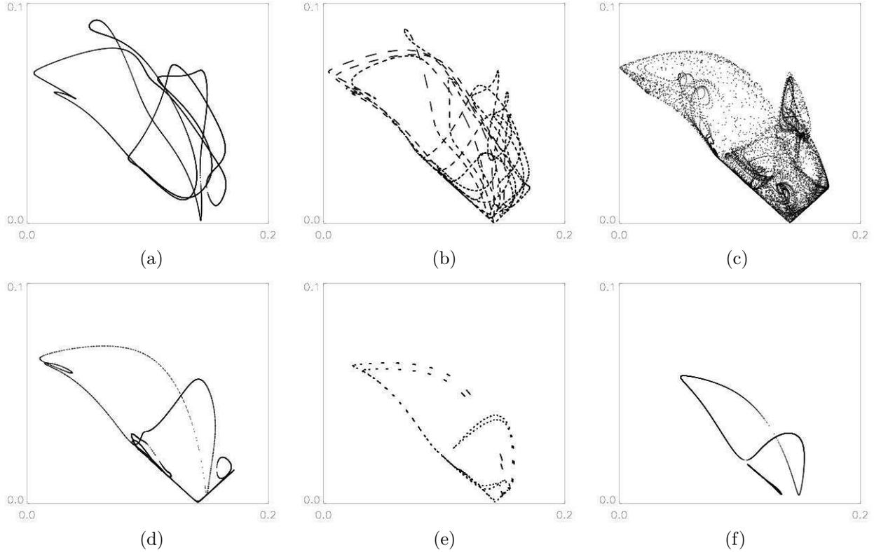
Figure 16: Poincaré sections for regimes in the family  $C^{SW}$  on the  $(|\hat{v}_{-1,2,1}^x|, |\hat{v}_{-1,2,1}^y|)$  quadrant (horizontal and vertical axes, respectively) defined by the condition  $|\hat{v}_{-1,2,1}^z| = 0.1$ :  $Ta = 80$  (a);  $Ta = 85$  (b);  $Ta = 90$  (c);  $Ta = 98$  (d);  $Ta = 102$  (e);  $Ta = 105$  (f).
