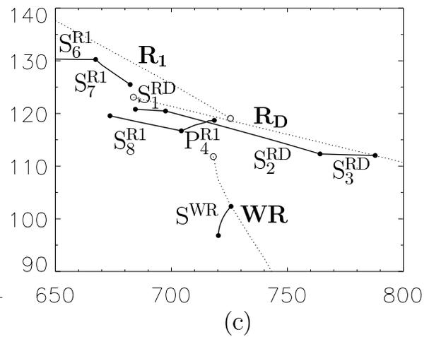
Figure 7: Kinetic  $E_k$  energy (vertical axis) of convective MHD attractors (solid line) and of hydrodynamic attractors (dashed line) for  $0 < Ta \leq 2000$  (horizontal axis). Labelling of attractors is explained in Sections 4 and 6 (see also Table 2).
