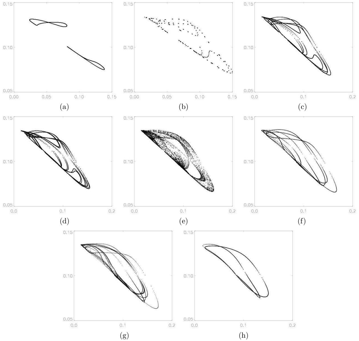
Figure 15: Poincaré sections for regimes in the family  $F^{TW}$  on the  $(|v_{-1,2,1}^x|, |v_{-1,2,1}^y|)$  quadrant (horizontal and vertical axes, respectively) defined by the condition  $|v_{-1,2,1}^z| = 0.2$ :  $Ta = 65$  (a);  $Ta = 70$  (b);  $Ta = 71.5$  (c);  $Ta = 72$  (d);  $Ta = 74$  (e);  $Ta = 77$  (f);  $Ta = 78.5$  (g);  $Ta = 80$  (f).
