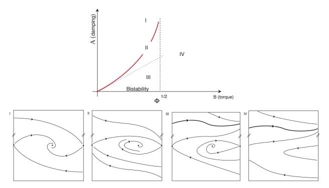
FIGURE 20. Top: bifurcation diagram for the pendulum with torque and corresponding phase portraits below. For parameters on the red curve II there is a homoclinic trajectory connecting two successive copies of the saddle. The thicker curve in regions III and IV is a closed trajectory on the cylinder.
