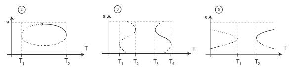
FIGURE 15. Schematic stability of fixed points of  $\mathcal{G}_T(s, y)$ , solutions of (6.16), in regions (2), (3) and (5) of Proposition 10. Conventions: solid lines are sinks, dashed lines are saddles, dotted lines are sources. Recall that y is a decreasing function of T. In region (2) the upper branch must undergo a bifurcation, indicated by an X, probably the Hopf bifurcation of Figure 14.
