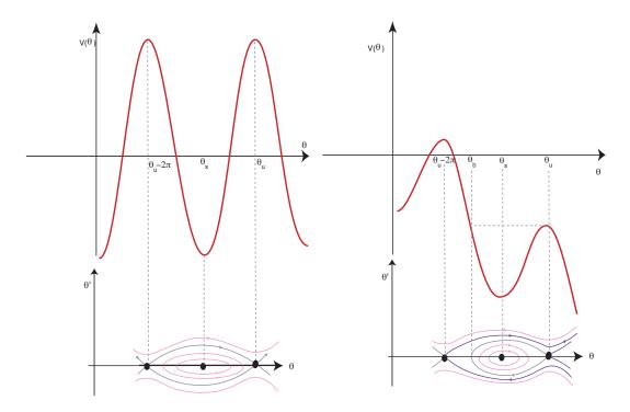
FIGURE 18. Phase portraits for the pendulum with no friction. Left: no torque, B = A = 0. Right: A = 0 and  $B \neq 0$ .
