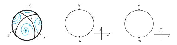
FIGURE 1. Sketch of the heteroclinic connections when  $\gamma = 0$  and  $\alpha > 0$ . When  $\alpha < 0$ , the arrows reverse orientation.
