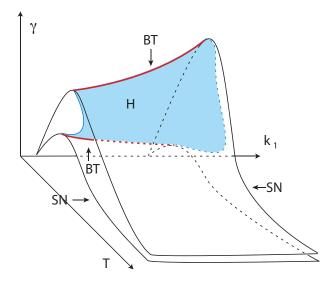
FIGURE 13. Schematic representation of the bifurcations of fixed points of  $\mathcal{G}_T(s, y)$  around the discrete-time Bogdanov-Takens, with  $k_1 < 1$ : the surfaces (a) of saddle-nodes SN (white) and the surface (b) of Hopf bifurcations H (blue) coming out of the red lines  $\gamma = M/(1-k_1)$ and  $\gamma = M/(1+k_1)$  of Bogdanov-Takens bifurcation points BT.
