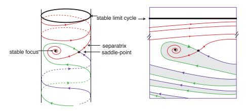
FIGURE 19. Phase portrait for the pendulum with torque, in a region of bistability. Right: the same phase portrait on a chart covering the cylinder. Points in the grey region have the stable focus as  $\omega$ -limit, trajectories of points in the white region go to the stable limit cycle.
